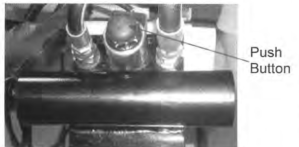
Figure 5-4. Push “Button” Lowering Valve
