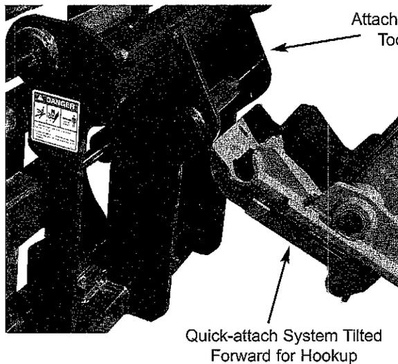
Quick-attach System Tilted Forward for Hookup
