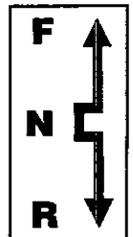
**NOTE:** The lever **MUST** be in N (Neutral) position before the starter will engage to start the engine.
