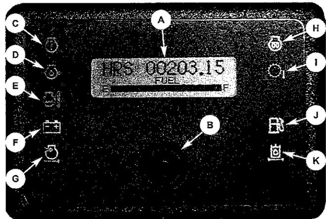
**A - Multi-Function Display Screen:** This screen displays the following functions:
