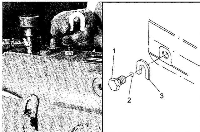
2. Turn the unlocking screws (1) fully in.
