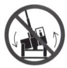
DO NOT use the frame leveling mechanism to compensate for swinging loads.
