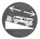
TETHER LOADS that may swing, keeping them close to the ground. Provide ample clearance for personnel to guide the load safely.
