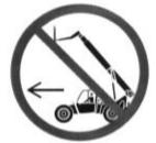
DO NOT operate on surfaces not capable of holding the weight of the telehandler; including the rated load (e.g., covers, drains, and trenches).
