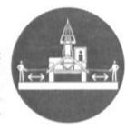
LEVEL FRAME ON SLOPES before elevating the boom.
