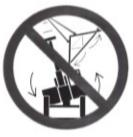
DO NOT enter the danger area under or around the boom when forks are off the ground or while engine is running.
