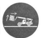
BE AWARE of the telehandler's travel envelope, especially when turning. Keep sufficient clearance at all times between the telehandler and any obstacles or people.
