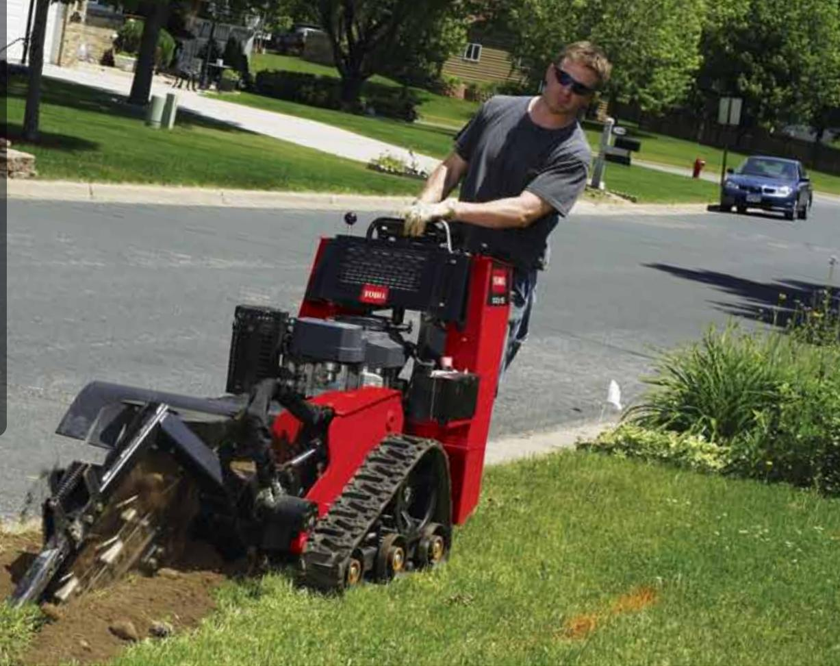
Easily bore under driveways and sidewalks to simplify irrigation and cable installations. Design allows for boring unit to be lowered into the trench to aid in level operation.
